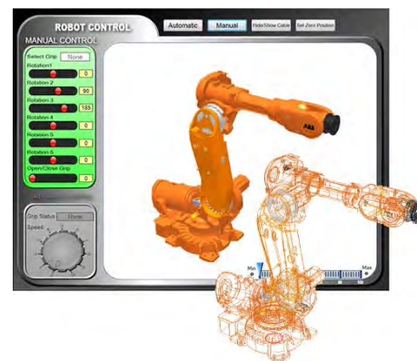
Fig. 14. 3D drawings imported in ICONICS HMI
